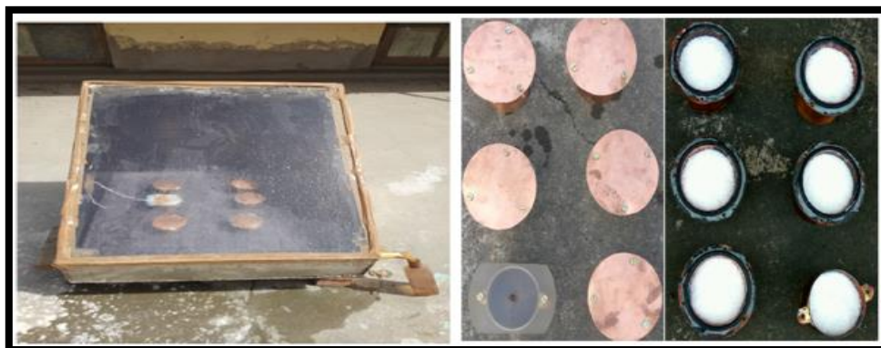
Figure: 25 Pictorial Representation of Single Basin Solar Still and Copper Cylinder Filled With PCM
