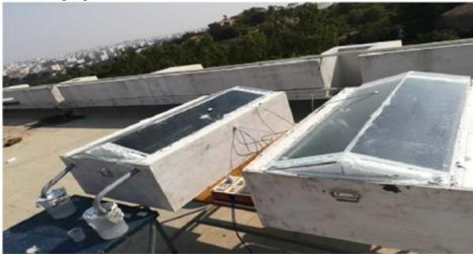
Figure 7: Depicts the Pictorial View of Experimental Setup with and Without Truncated Conic Fins
