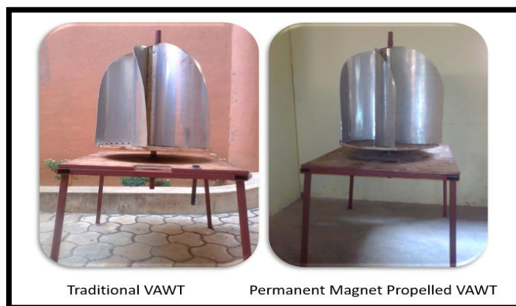
Figure 4: Conventional VAWT Model vs PM-VAWT Model
