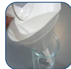
C – Calcium oxalate ppt filtered,
