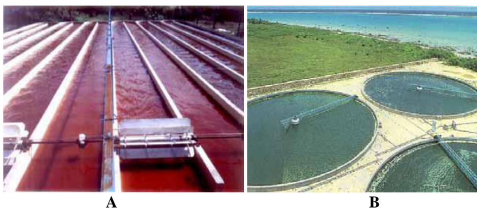
1. H. pluvialis production in raceway paddle wheel mixed ponds (Parry Nutraceuticals, India).
