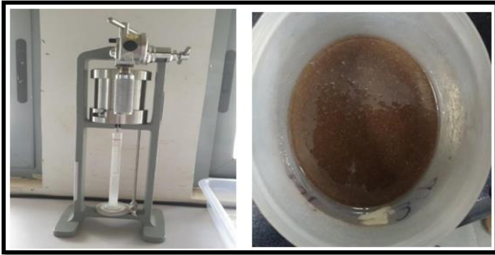
Figure 4: LPLT Filter Press
