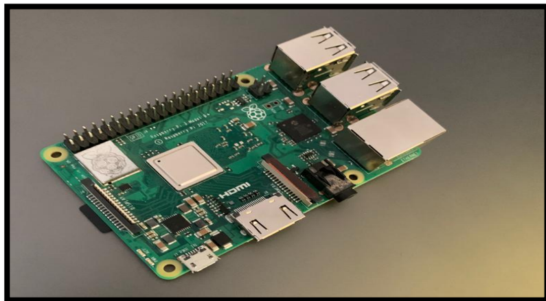
Figure 2: Raspberry - Pi 3 B+
