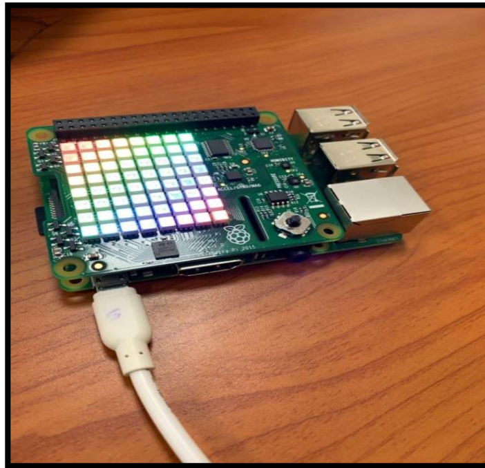
Figure 3: Raspberry-Pi Sense HAT
