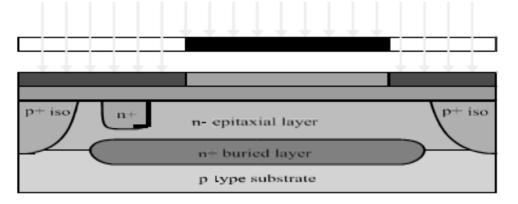
**18. Base area implantation:** Implantation is performed into the epi layer using a p type impurity (usually boron) through the oxide window and p type base region is formed.
