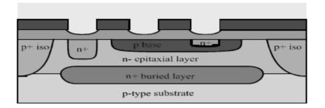
**23. Final contact cuts after etching:** Openings have been created in the oxide layer which will allow access to the collector, base and emitter regions.
