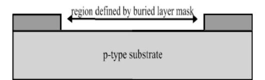
**6. Implant of buried layer:** The buried layer is fashioned with a excessive density (dose) implant of n-type dopant, typically phosphorous. A few lateral diffusion of dopants takes area in the course of the implant. Dopant is also brought into the overlaying oxide.
