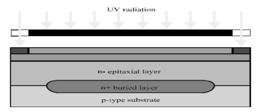
**11. Isolation implantation:** A heavy p-type doping through ion implantation forms the p+ isolation regions. Implantation between the isolation regions is prevent by masking oxide which absorbs dopant.
