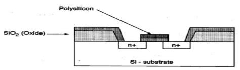
**Step 8**:  $SiO_2$  and photoresist is again deposited on the source and drain terminals: The process in step 6 is again repeated to protect the source and drain terminal. The oxide layer is etched from the surface of the wafer so that the two terminals can be created. The SiO2 and photoresists are deposited and photolithography process is repeated. The contact holes area are left exposed and space for connection are left behind.
