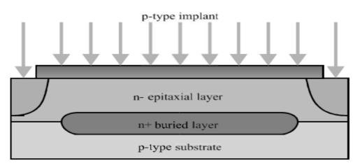
**12. Final isolated structure:** Once the isolation reaches the underlying substrate the masking oxide is removed.
