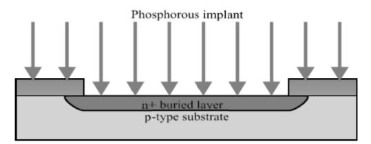
7. The final buried layer: After the overlaying oxide is eliminated (etched), the result is a surprisingly doped buried layer place in the unique silicon substrate.
