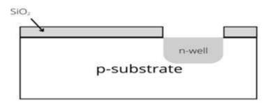
7. **Removal of SiO<sub>2</sub>:** The remaining oxide on the surface of the wafer is etched with the help of Hydrofluoric acid (photolithography process is repeated).
