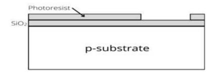
**5.** Oxide etching: As we saw in the previous figure the right side of the wafer is not covered by the photoresist. Since we have to form a n-well in this part we will etch the oxide layer using Hydrofluoric acid. So, along with the oxide layer the remaining photoresist will also be etched. Now, our silicon wafer is ready to get dopped in the n-well area.
