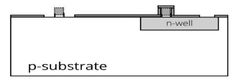
**12. N-diffusion regions:** The two vacant areas mentioned above include two source terminals and two drain terminals on each side. The N-diffusion regions are produced either by diffusion or ion implantation process. Now, the source and drain terminals are automatically formed on the adjacent sides of the gate terminals. During this process the wafer is heated to a high temperature to create a n-well regions through the diffusion process.
