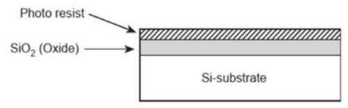
**Step 4**: Process of Photolithography: The photoresist layer deposited in the previous step is now exposed to ultraviolet radiation. For this a mask is created. Mask determines the regions through which the diffusion will takes place. The mask will split into two regions, one which is covered and another which is exposed to UV radiation. The areas which get exposed by UV radiation becomes polymerized (hardened). The areas where diffusion process will take place are guarded by the mask.
