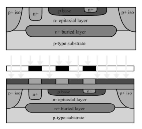
**22. Contact etching:** This openings requires selectivity so etching process does not remove emitter region, therefore wet Chemicals used.
