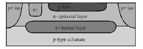
Now the Emitter Region Exposure PR layers are exposed using an emitter mask on the glass plate.
