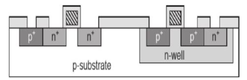
**15. Metal formation:** Now, evaporated aluminium is coated on the surface of the wafer. This forms a metal layer on the surface of the wafer. Now, patterning (photolithography) is done to obtain the contact holes.
