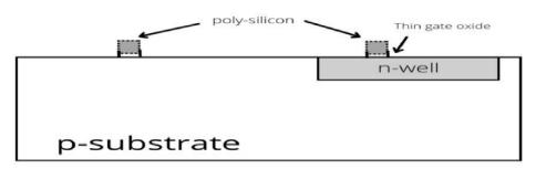
**10. Diffusion pattern:** The entire surface of the wafer is covered by a protective thin layer of the oxide. The purpose of this thin layer is to protect the two gate terminals.
