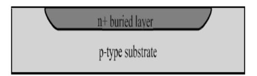
8. Deposition of epitaxial layer: Using epitaxial deposition (just like CVD), a layer of very excessive high-quality (crystalline) silicon is deposited at the surface. Some diffusion of dopants happens from the tremendously doped buried layer into the greater lightly doped epitaxial layer.
