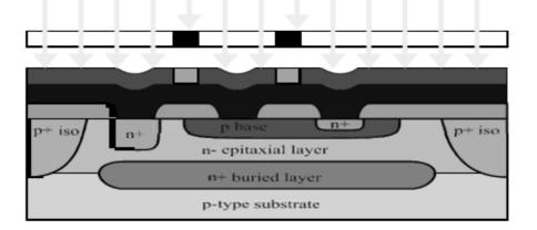
**25. Final interconnect structure:** As the metal has been etched to form the interconnections between contacts, the final structure is complete. The Modern processes would use more than one layers of metal.
