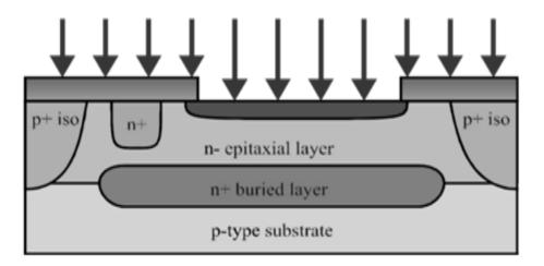
**19. Final base region:** After base area implantation is complete, a counter doped base region has been created in the n-type collector.
