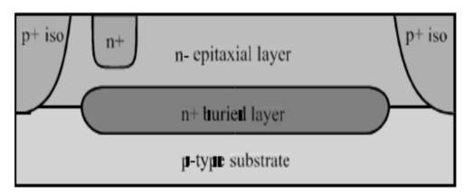
**17. Base mask publicity:** The oxide is formed and the region in which active base has to be formed is exposed using the base mask.
