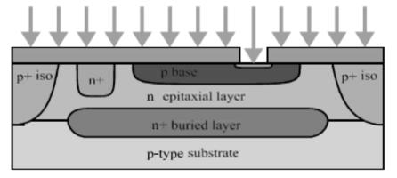
**21.** At the end emitter structure and contact cut exposure: N<sup>+</sup> emitter region in the p-base completes the basic BJT structure, only metal contacts remain. Now thin Oxide is deposited which will isolate metal connections. Photo Resist is exposed using contact cut mask.
