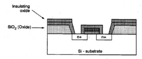
**Step 9:** Deposition of Metal layer: This is the last step of the NMOS fabrication process. A layer of evaporated aluminium is spreaded on the surface of wafer including the contact holes. This aluminium layer is around 1um thick. The metallic layer is again masked and etched (photolithography) to form the desired interconnection pattern.
