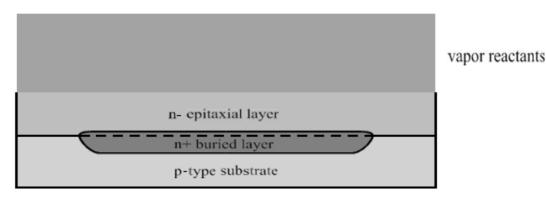
**9.** The final Epitaxial Layer: The resulting epitaxial layer will shape the collector location within the BJT, with the highly doped buried layer forming an equipotential region under the device. The buried layer is now completely enclosed in silicon fabric. 4
