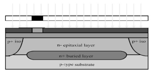
**15. Sinker implantation:** N type impurities are implanted into the window etched in the oxide to form a sinker.
