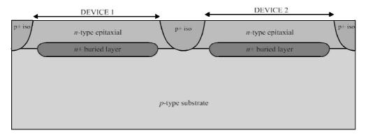
**14. Sinker mask exposure:** Connection may be made to the buried layer (collector) by usage of a sinker, an implantation of high concentration and significant depth. Oxide and PR layers are exposed through a sinker mask.
