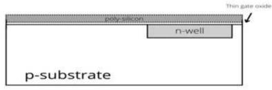
**9. Patterning of poly silicon layer:** As we know CMOS is a combination of PMOS and NMOS, so we need two separate gate terminals. To obtain these two separate gate terminals photolithography process is repeated. The two gate terminals which are formed are shown below in the figure.
