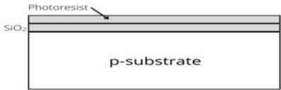
4. Formation of N-well: At this stage, the photoresist material is highly insoluble so we place a mask over the substrate covered by  $SiO_2$  and photoresist layer. Through this n-well mask uv light is exposed (photolithography).
