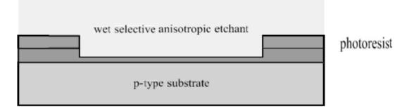
5. The final buried layer window: After the left over photoresist is stripped, the deposited oxide has an opening etched within the location provided by the buried layer mask.
