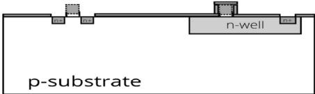
**13. P-diffusion:** In the earlier step, the n<sup>+</sup> regions are already created and since NMOS has n<sup>+</sup> source and drain regions while the PMOS has p<sup>+</sup> regions. Now, the p<sup>+</sup> diffusion mask is used (photolithography) which completes our formation of all the active regions of the MOS transistors.
