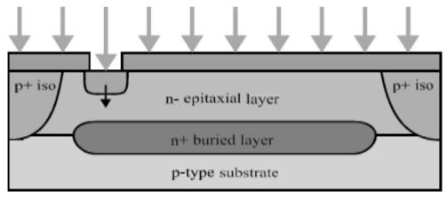
**16. Final sinker structure:** Whether the sinker will reach down the buried layer or not depends on the condition of the implantation and thickness of the buried layer.
