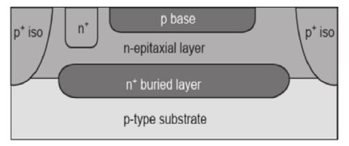
**13. Illustration of p^+ isolation:** Through connecting to the underlying substrate, the p+ isolation implants electrically disconnect regions of the epi layer from every other. The pn junction formed between the p+ implants and the n type epi layer provides the isolation electrically.
