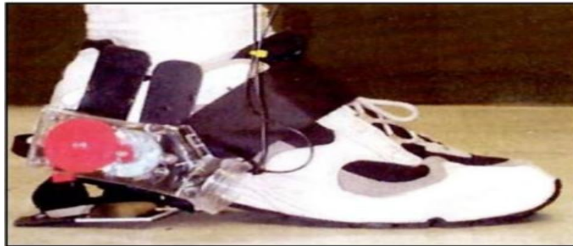
Figure 5: Magnetic Generator Adapted in a Shoe
